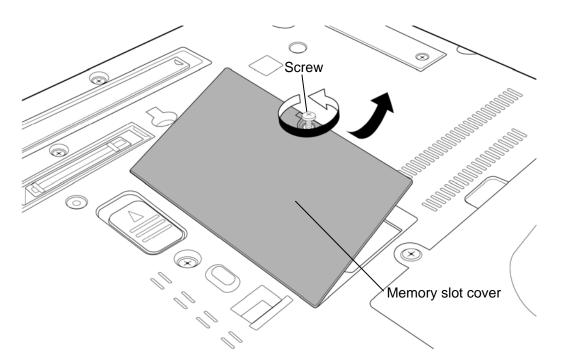
Figure 4-11 Removing the memory slot cover (slot B)
